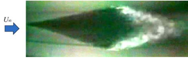
Fig. 2 Turbulent spot visualization at high free stream turbulence, Tu = 0.01\% of U_\infty (Allfredsson et al. 1996)
